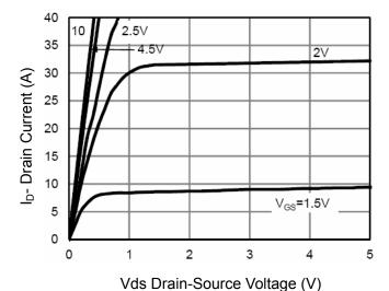
**Figure 5 Output Characteristics**
