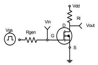
**Figure 1:Switching Test Circuit**
