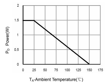
**Figure 3 Power Dissipation**
