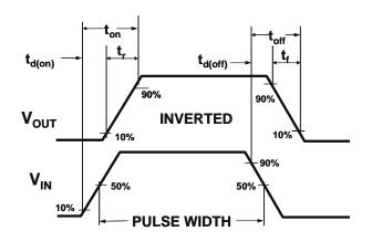
Figure 2:Switching Waveforms
