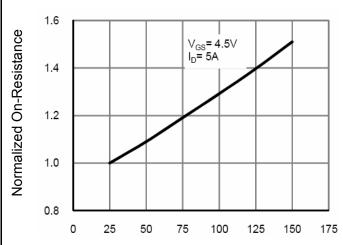
Figure 8 Drain-Source On-Resistance
