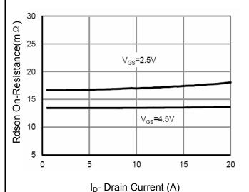
Figure 6 Drain-Source On-Resistance
