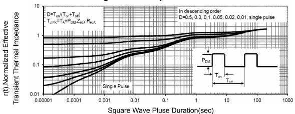
**Figure 14 Normalized Maximum Transient Thermal Impedance**
